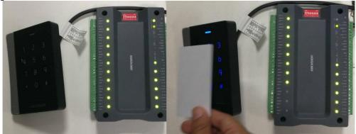
I give this card the permission of the first three floors, after swiping card, We can see the corresponding relay acted by these pictures $_{\circ}$
