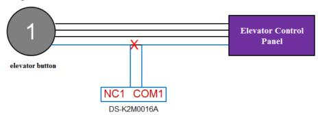
After the authentication is passed, the relay closes and the button enables
