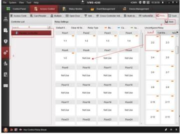
**Note**: Drag the right relay to the corresponding floor
